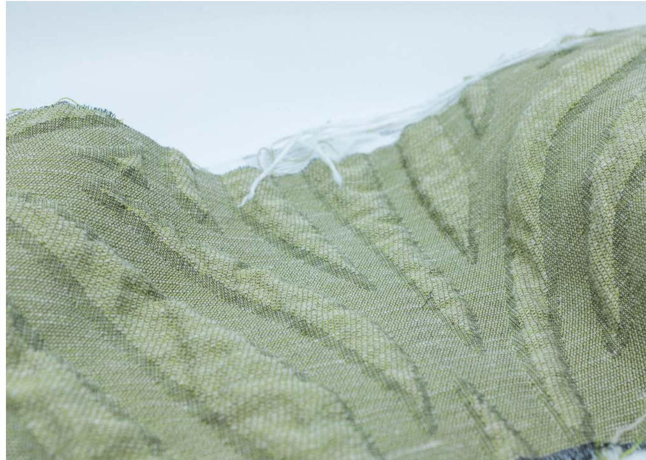
Open pocket structures with thicker wadding weft results as heavy three-dimensional matelassé fabric used in bed covers / image by Petra Haikonen
