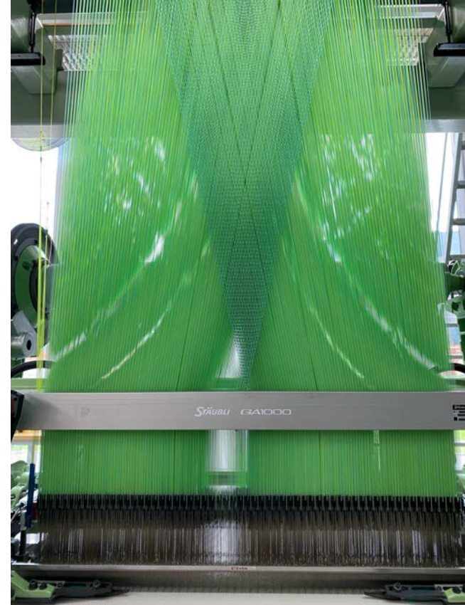
Industrial rapier machine with a 2 repeat jacquard harness where one hook operates 2 heddles simultaneously / image by Petra Haikonen
