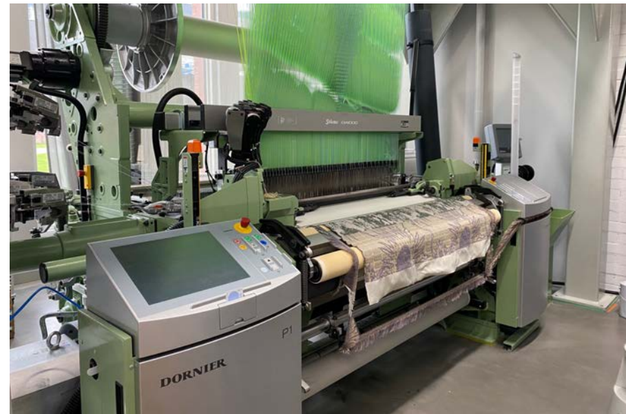
Industrial rapier machine with jacquard harness at Aalto University, Espoo / image by Petra Haikonen
