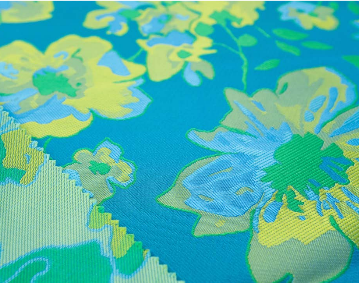
This double-faced fabric is woven with one warp yarn (blue) and three weft yarns (light blue, green & yellow) / image by Petra Haikonen
