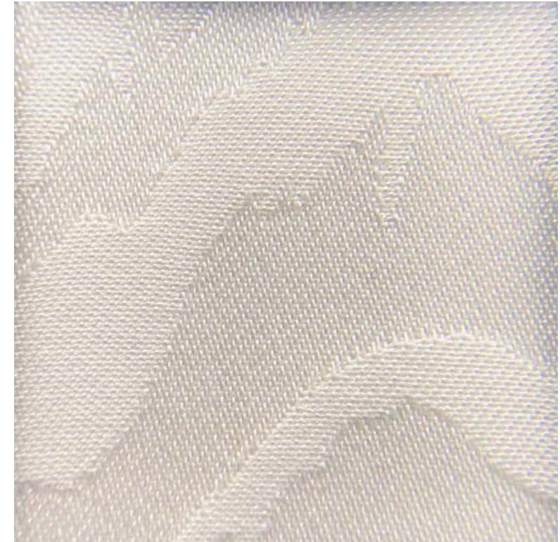
Close-up image of damask with warp-faced and weft-faced satin structures / image by Petra Haikonen
