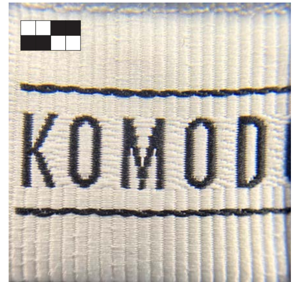
Close-up images warp- faced rib (top) and weft-faced rib for Komodo's shirt label (bottom) / images by Petra Haikonen
