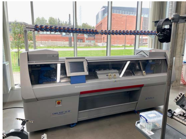
Stoll's ADF flat-bed weft knitting machine at aalto University in Finland / photo by Petra Haikonen
