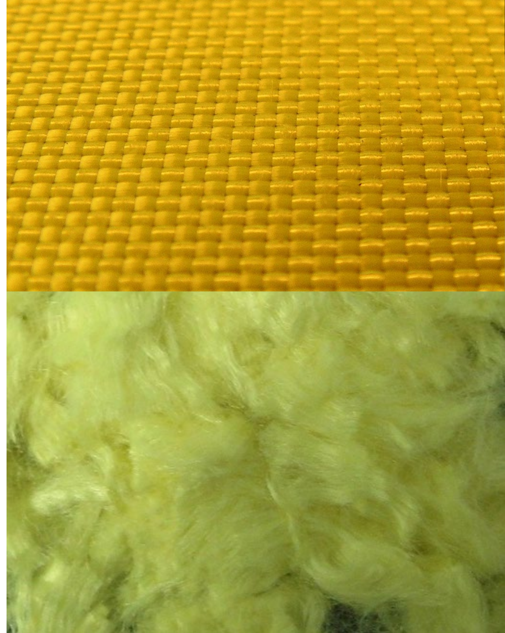
Aramid fabric, photo by No-w-ay on Wikipedia CC BY-SA 4.0 Kevlar staple fibre, photo by Cjp24 on Wikipedia CC BY-SA 3.0
