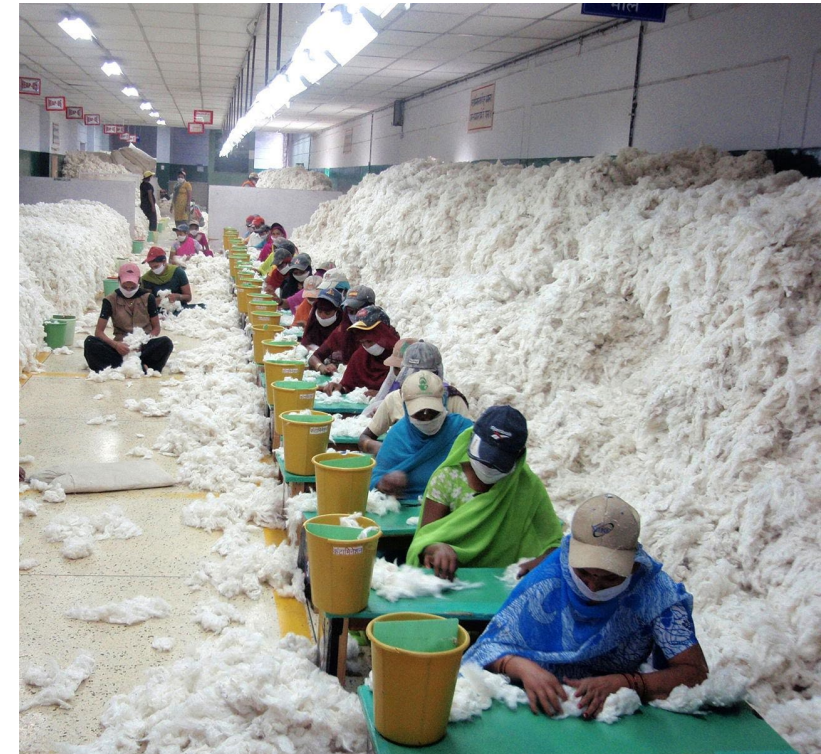
Manually decontaminating cotton before processing at an Indian spinning mill, photo by CSIRO on Wikipedia, CC BY 3.0 DEED
