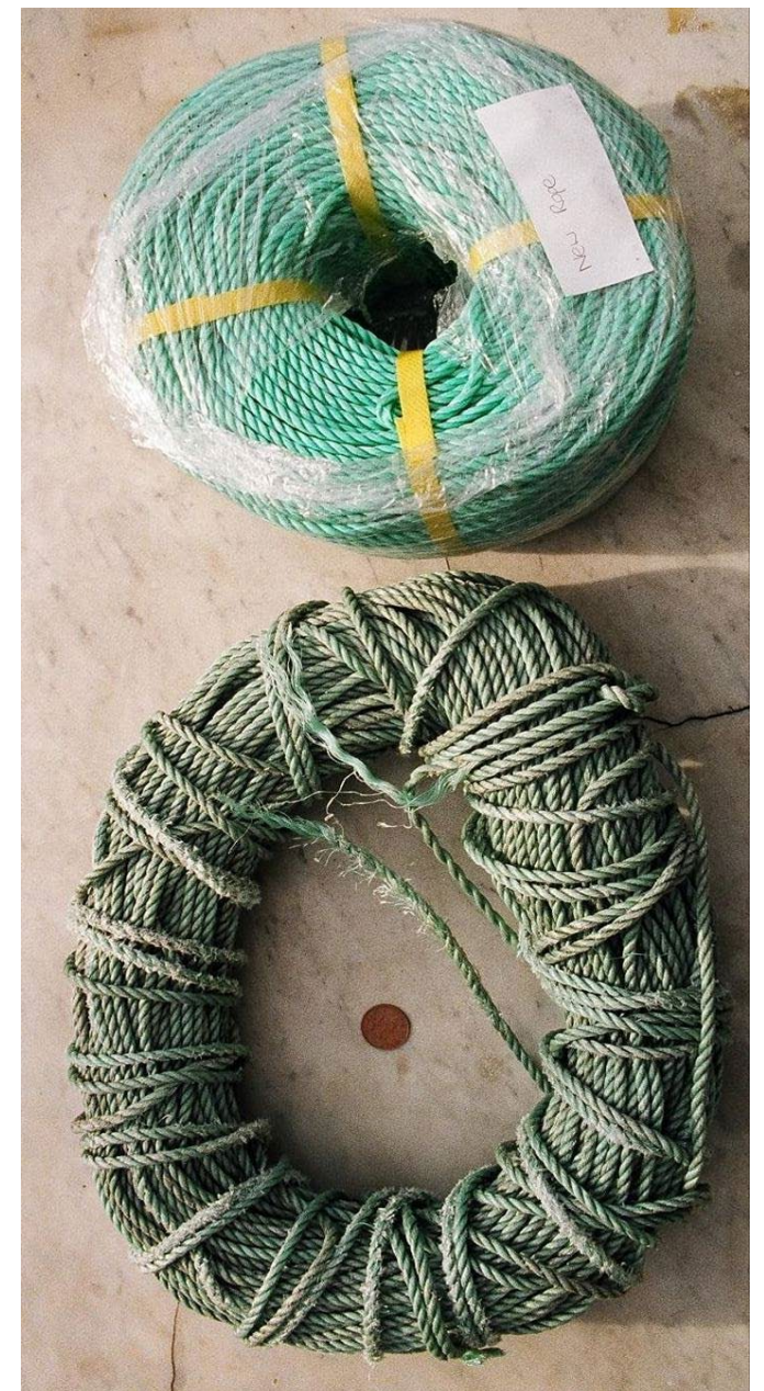
Effect of UV exposure on polypropylene rope. Photo by Peterlewis on Wikipedia (Public domain)
